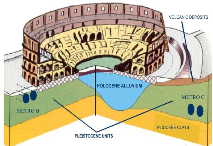
Block diagram of the Coliseum showing the underlying geology and the occurrence of unconsolidated Holocene alluvial deposits which have caused the collapse of half of the external walls due to differential shaking during the 1349 earthquake (Funicello et al., 1995).
