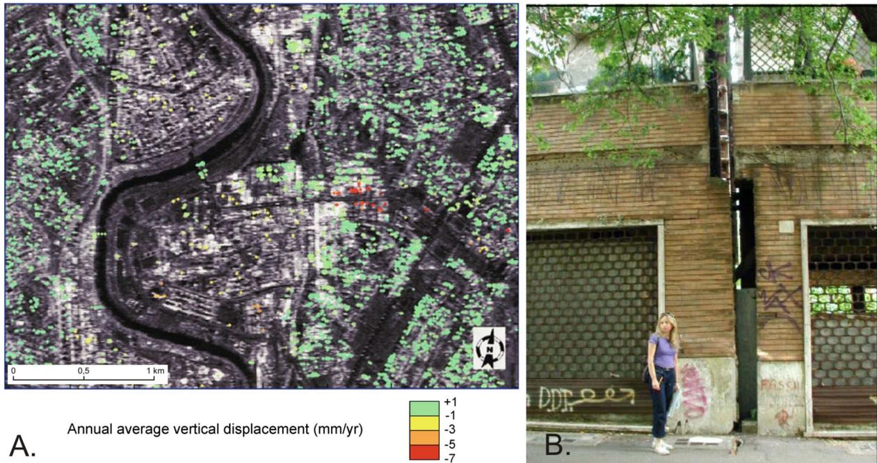
A. Estimate of vertical displacement of building from multi-image radar map analysis (from Giordano, Mazza et al., 2004). At present, several edifices built over unconsolidated clays are monitored from selective subsidence. This image is a courtesy of F. Ferrucci and has been obtained by comparing 10 years of satellite images. B. Evidence of differential subsidence on the structure of buildings.
