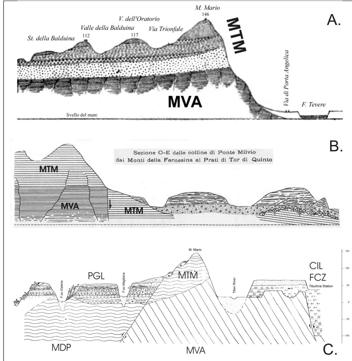
The three sections show the tectonics and the unconformity relationships between the Pliocene Monte Vaticano Fm. and the Lower Pleistocene Monte Mario Fm. A. Tellini (1896); B. Verri (1915); C. Conato et al. (1980).
