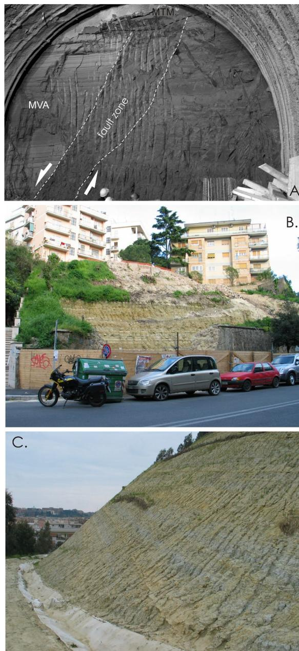
A. The unconformity between the Pliocene marine clays (MAV) and the Lower Pleistocene silts and sands (MTM) exposed during the excavation of the Galleria Giovanni XXIII through Mt. Mario. Note the tectonic deformation sealed by MTM; B. The MAV clays and sand crop out along the Mt. Mario slopes, seldom causing landslides (Via Labriola); C. Excavation of the MAV clays at Via di Donna Olimpia for the construction of an underground parking, needs special care for the presence of nearby housings.
