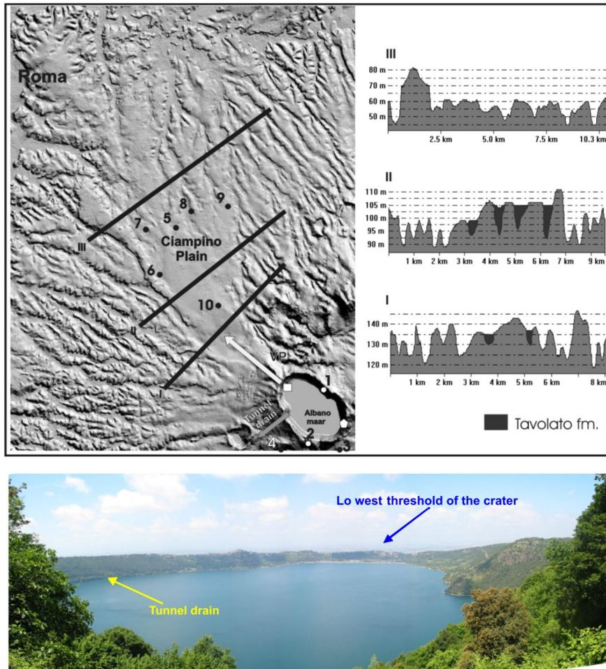
A. profiles across the Ciampino plain show the Holocene infilling of the Last-Glacial fluvial network by the lahar deposits of the Tavolato Fm. (from De Benedetti et al., 2008); B. View of the Albano lake with the location of the tunnel drain built by the Romans to keep the lake level 70 m below the lowest threshold of the crater rim, in order to prevent further overflows, the last having occurred in 398 B.C.E.
