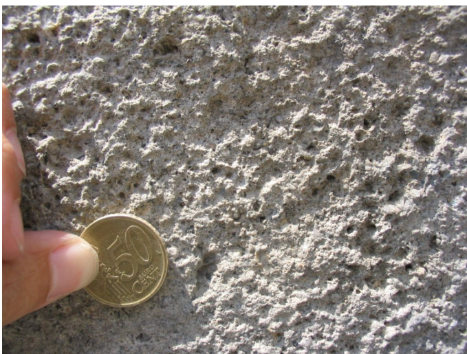
Figure 63. Weathering of the Phlegrean lavas.
