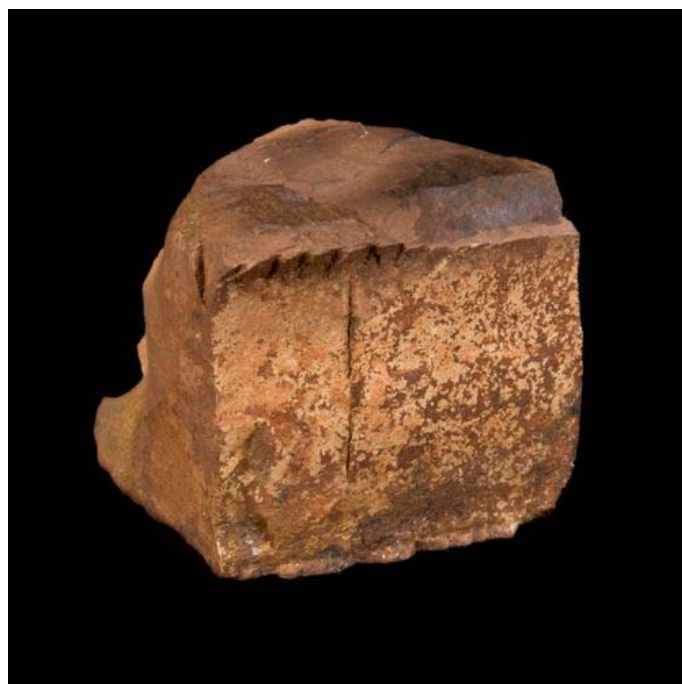
Figure 12. Photograph of jointed specimens of bedded chert from the Chert Series Beds
