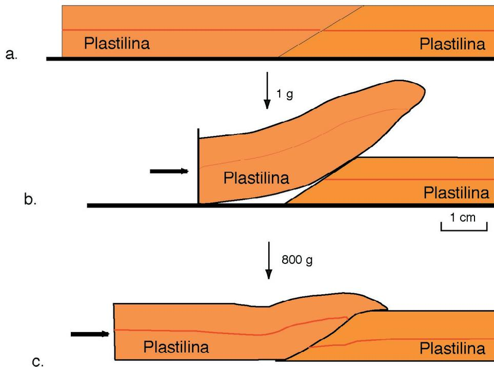
**Figure 4.** a) Initial set-up of a single plastilina layer detached above a rigid base. b) and c) represent deformed models under normal gravity and in a centrifuge, respectively.
