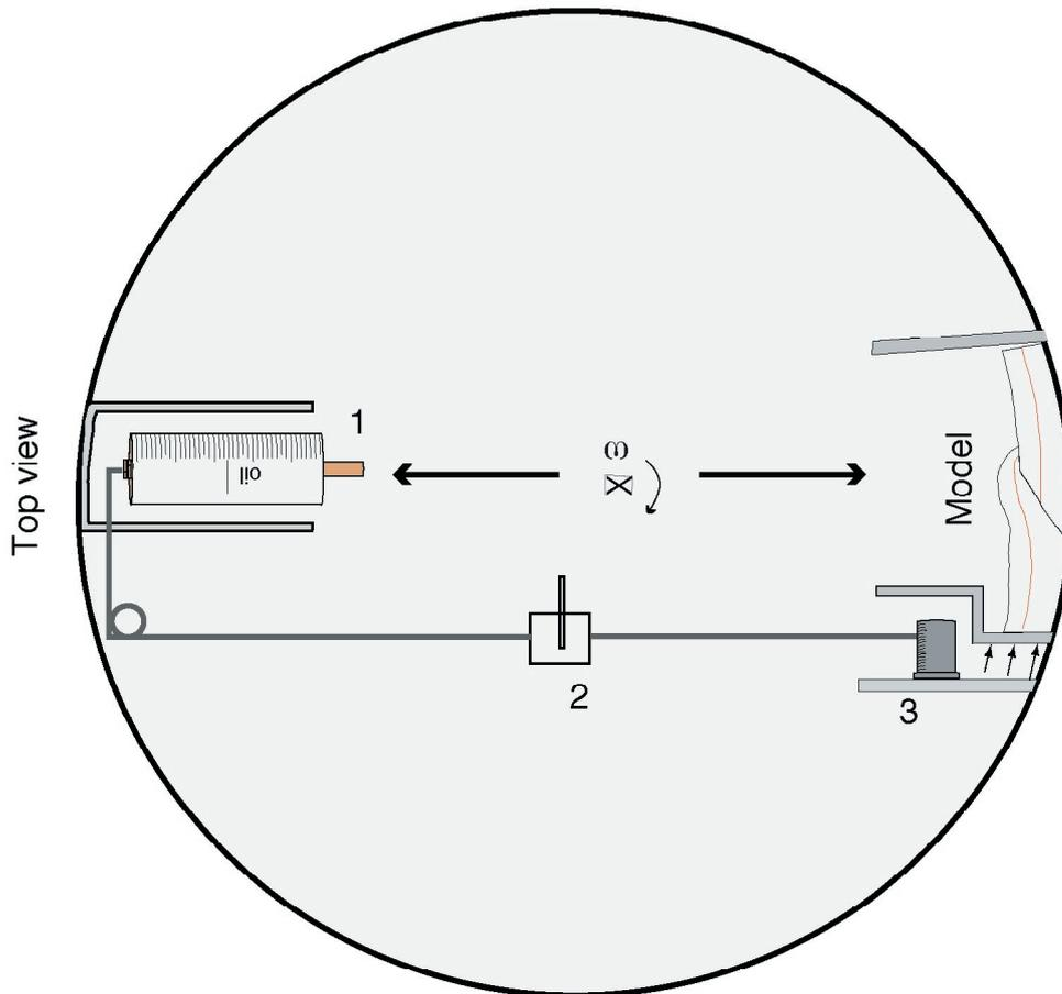
**Figure 2.** Diagrammatic representation (not to scale) of top view of a hydraulic squeeze-box used to deform models in a centrifuge. 1. Hydraulic cylinder. 2. Magnetic valve used to switch on and off the compression. 3. Telescopic cylinders pushing the rear wall of a squeeze-box.
