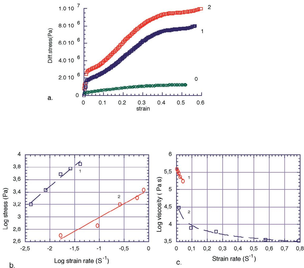
**Figure 3.** a) Stress-strain behaviour of plastilina at different confining pressures ( 0, 1 and 2 in MPa, respectively). b) Stress-strain rate behaviour of hardened (1), and softened (2) DC 3179 dilatant compound, used to simulate the incompetent surroundings in nature. c) Viscosity versus strain rate curves showing the strain rate softening behaviour of the incompetent surroundings.
