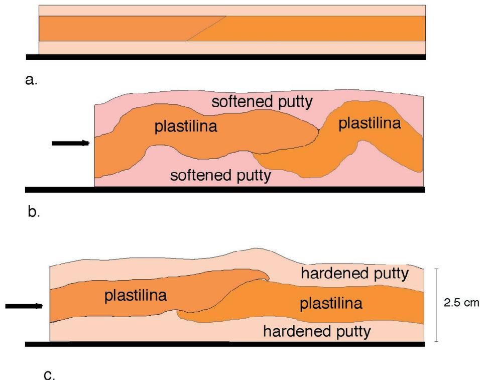
**Figure 7.** a) Initial set-up of three-layer models where the competent single layer is sandwiched between soft (b) and stiff (c) ductile strata.
