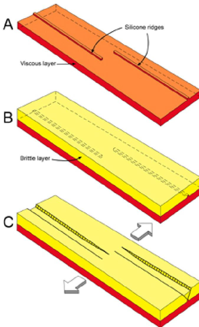
Experimental set-up used by Le Calvez and Vendeville (2000) to model graben relays using a thick layer of viscous silicone overlain by a thick sand layer. Two narrow ridges of silicone at the base of the sand layer trigger nucleation of two offset grabens.
