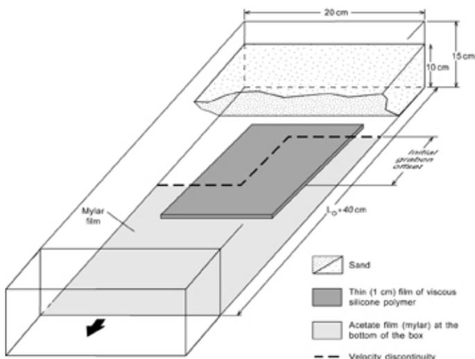
Experimental set-up used by Le Calvez and Vendeville (1996) to model graben relays using a sand layer, a weak basal viscous layer, and a basal plastic sheet. Note that only the center of the model comprises the weak viscous layer.
