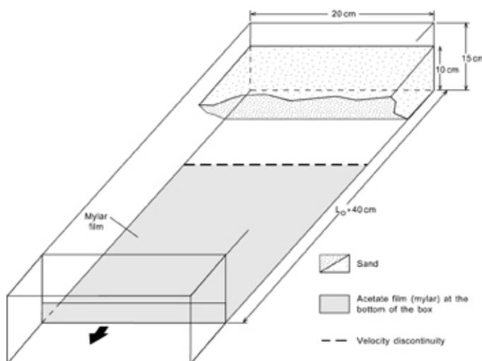
Experimental set-up used by Faugère and Brun (1984) to model pure extension using a sand layer resting on a basal plastic sheet.
