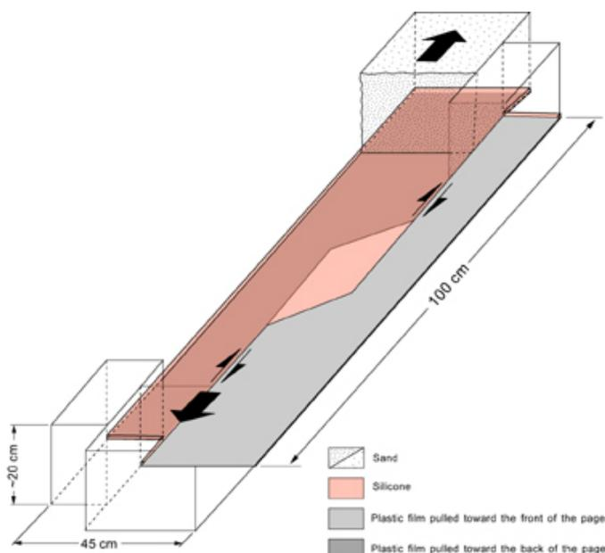
Experimental set-up used by Sims et al. (1999) to model pull-apart basins using a sand layer, a strong basal viscous layer, and a basal plastic sheet.
