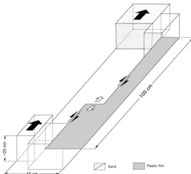
Experimental set-up used by Faugère and Brun (1984) to model pull-apart basins.
