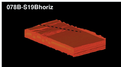
Figure 20. Structures in experiment 078 after 15% extension during second rifting event, illustrated by surface photograph, vertical sections and three cut-out 3-D perspective views.
