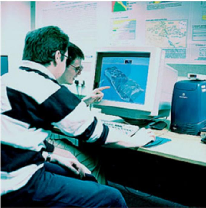
Photogrammetric mapping of 3-D digital models in action by team members. The models once completed can be viewed in stereo by use of a Nu-vision screen and polarised glasses, and can be freely rotated and viewed from any desired orientation.
