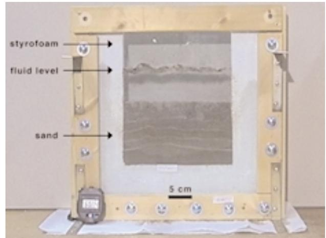
**Figure 1.** Glass tank that was used for the segregation experiments. The simple set-up consists of a wooden frame that holds together two glass plates that are separated by styrofoam, to create a 1.5 cm wide sample chamber. Ascent experiments were carried out in a similar, but larger tank.
